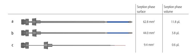
Immersion Extraction: Polyaromatic Hydrocarbons (PAHs) in Water
