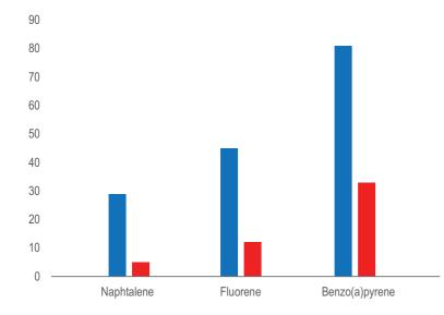
Relative immersion extraction yield (measured as % extracted after a 70 min) for PAHs at 50 ng/L with PDMS fibers (PAL SPME Arrow 100 µm, 20 x 1.1 mm compared to SPME 100 µm, 10 x 0.3 mm)
