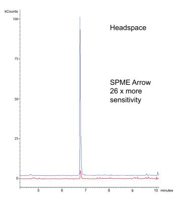
Extraction of 1 µg/L iodoform from tap water with DVB fibers (headspace and immersion extraction), PAL SPME Arrow 100 µm, 20 x 1.1 mm compared to SPME 100 µm, 10 x 0.3 mm.
