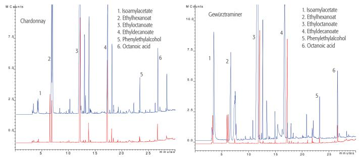
Chromatograms showing the headspace extraction of aroma components from different white wines with PDMS fibers (PAL SPME Arrow 100 µm, 20 x 1.1 mm compared to SPME 100 µm, 10 x 0.3 mm)
