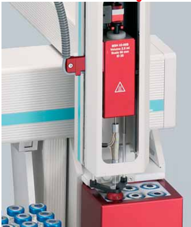
ITEX adsorption step out of a sample vial
