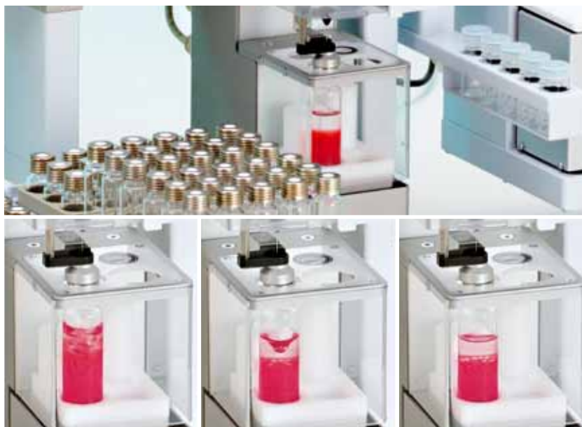
Vortex Mixer showing fully automated Liquid / Liquid Extraction Process
