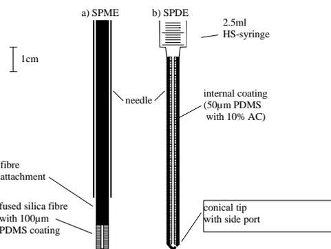
Fig. 1: Schematic representation of the SPME device (a) in comparison to the SPDE device (b)
