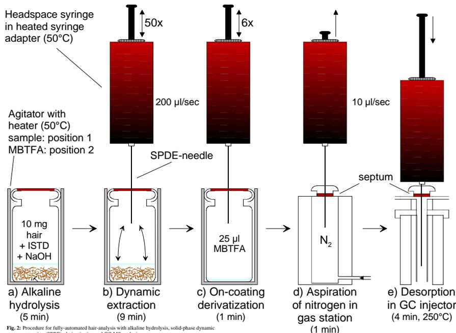
Fig. 2: Procedure for fully-automated hair-analysis with alkaline hydrolysis, solid-phase dynamic extraction (SPDE), derivatisation and GC-MS analysis.
