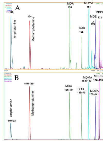
Fig. 4: Chromatograms of spiked hair samples (0.5 ng/ml) measured using the Q1-SIM mode (A) and the MS/MS multiple reaction monitoring mode (B)
