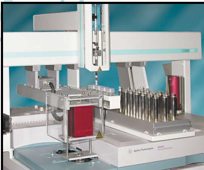
Fig. 1. Thermal desorber option attached to CTC PAL using an Agilent 6890 GC
