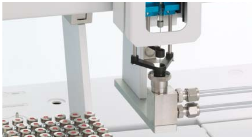
Flow-Through Cell for online analysis
